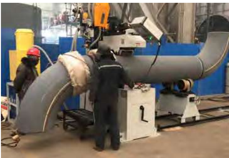
SAW process for fill and cosmetic welding
