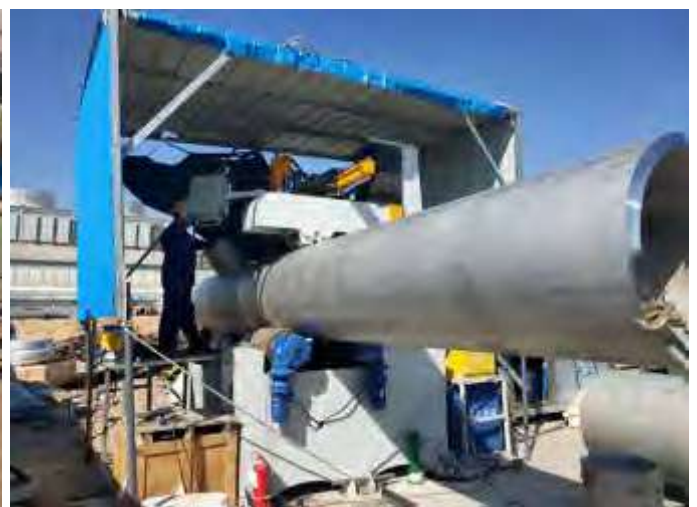
SAW process for fill and cosmetic welding
