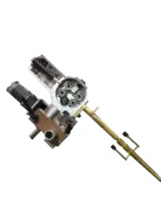
Visible arc cladding
