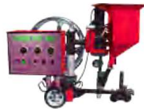
Pipeline welding tractor
